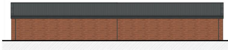
Six Bay Garage - Rear Elevation
